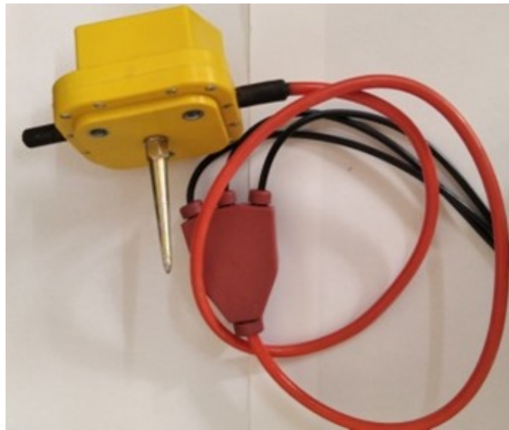
Figure 4. Three-axis geophone with cutoff frequency f_c = 4.5 Hz.
